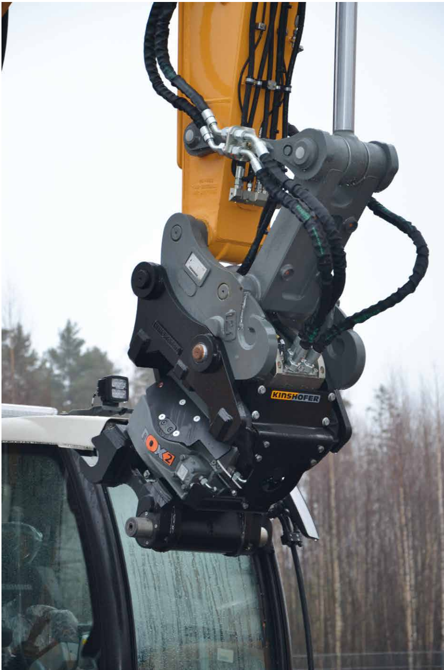
“The most advanced Tiltrotator in the world” NOX equipped with Likufix upper bracket and Liebherr SW48 lower quick coupler
