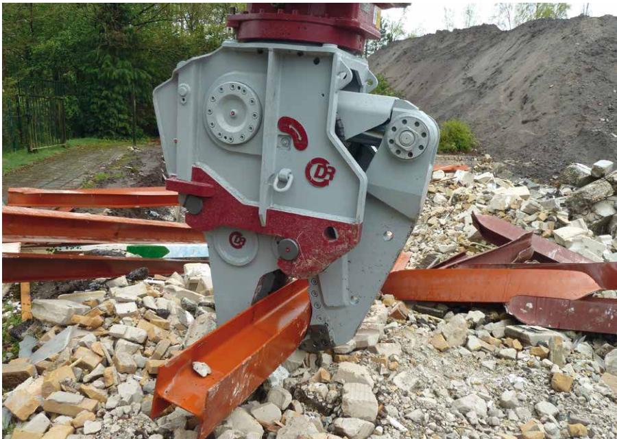
MQP-S with steel cutting jaws
